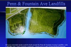
100 acres intertidal marsh could be built around the Penn & Fountain Avenue Landfills with 1,500,000 cubic yards of dredge sediments, cement lock or other treated dredged material, and/or rock blasted from harbor deepening .
